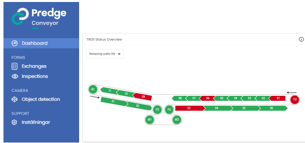
Figure 3. Side view menu of dashboard and belt status overview. The idlers are sectioned appropriately to prevent from cluttering. Each section contains 50 idler sets, that is left, center, right roller each.
