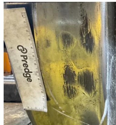
Figure 3 Multiple wheel flats on a single wheel
