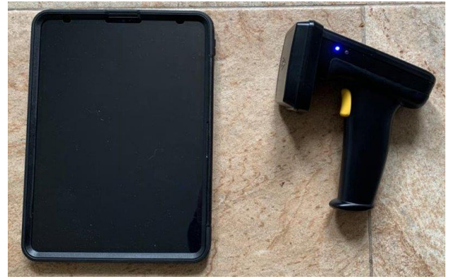
Figure 2 RFID reader and tablet used for workshop data collection
